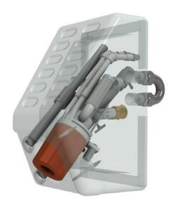
The JetBOx™ is designed to position the burner and oxygen injection as close to the steel bath as possible for the highest injection efficiency with no fear of damage to the EAF as it provides excellent cooling protection and is capable of withstanding the impact of falling scrap and splashing of slag and molten metal.
